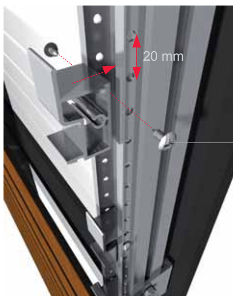
INSTALLATION OF BASE PART
