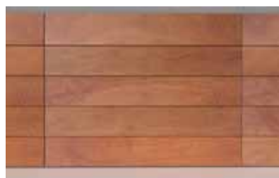
STAGGERED PATTERN IN MULTIPLES OF 600mm.
